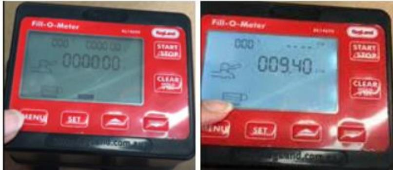
2. Press SET for 3 seconds and use the up and down arrows to set the pin number to 1234 (default password)
